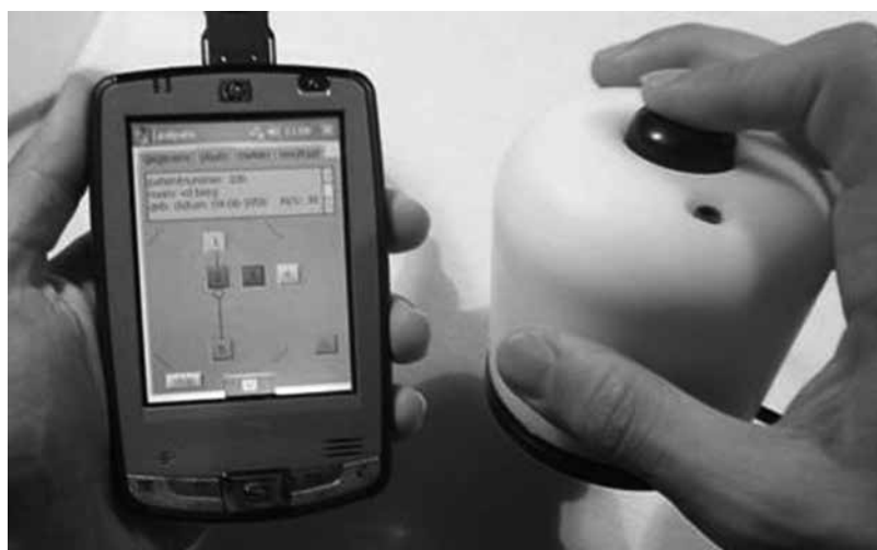
Figure 6. Tensiometer to measure abdominal compliance and pressure. The new prototype used for measuring AWT consisted of a built-in force and distance sensor, attached to a handheld personal digital assistant (PDA, HP IPAQ). The diameter of the circle-shaped base of the device is 72 mm. The tip of the instrument is shaped like one half of a sphere and has a diameter of 18 mm, with a total surface area of approx. 5.1 cm 2 . The shape of the tip was chosen due to the extensive use of this shape in industrial hardness measurements of materials. The size of the tip was chosen due to its comparability to the conventional instrument by which abdominal tension is estimated, which is the human finger. This device can measure the amount of force (N) needed to indent a certain distance (mm), which is then visualised on the PDA in graphics (adapted from [34])
