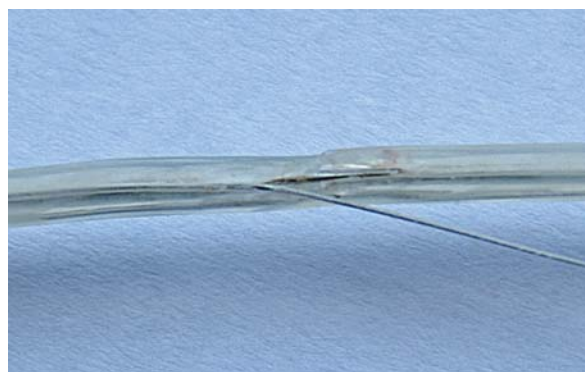
Fig. 3. Defibrillation lead failure – an insulation and inner leads defect is clearly visible
