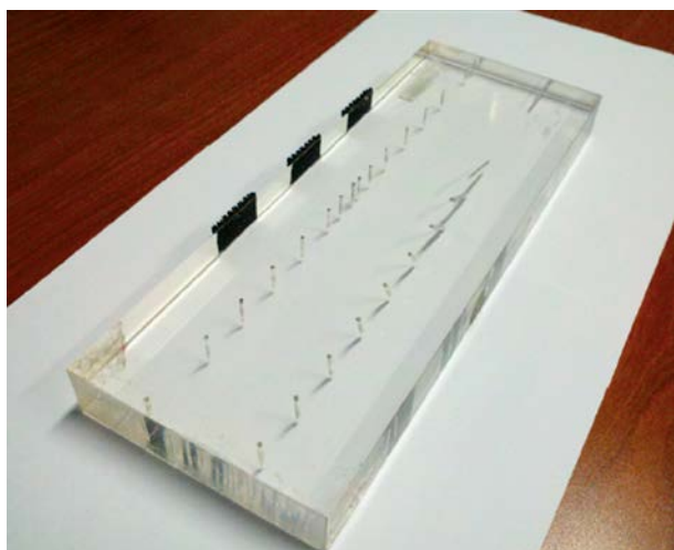
Fig. 4. Publications report using polycarbonate support used in the orientation accuracy analysis. The support contains machined holes with predefined orientations ( \pm 1^\circ )
